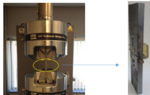
Figure 4 Specimen mounted between the jaws of Universal Testing Machine.
