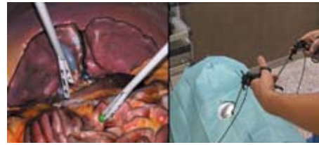
Figure 8 ULIS patient-specific laparoscopic simulator. Our R&D department is working on the development of an AR-based simulator named ULIS (Unlimited Laparoscopic Simulator) which integrates the 3D patient-specific anatomical model with haptic feedback based on texture and tissue resistance providing the surgeon highly realistic images and haptic feedback.
